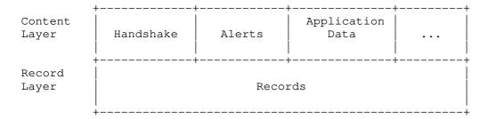
Figure 1: TLS Layers
