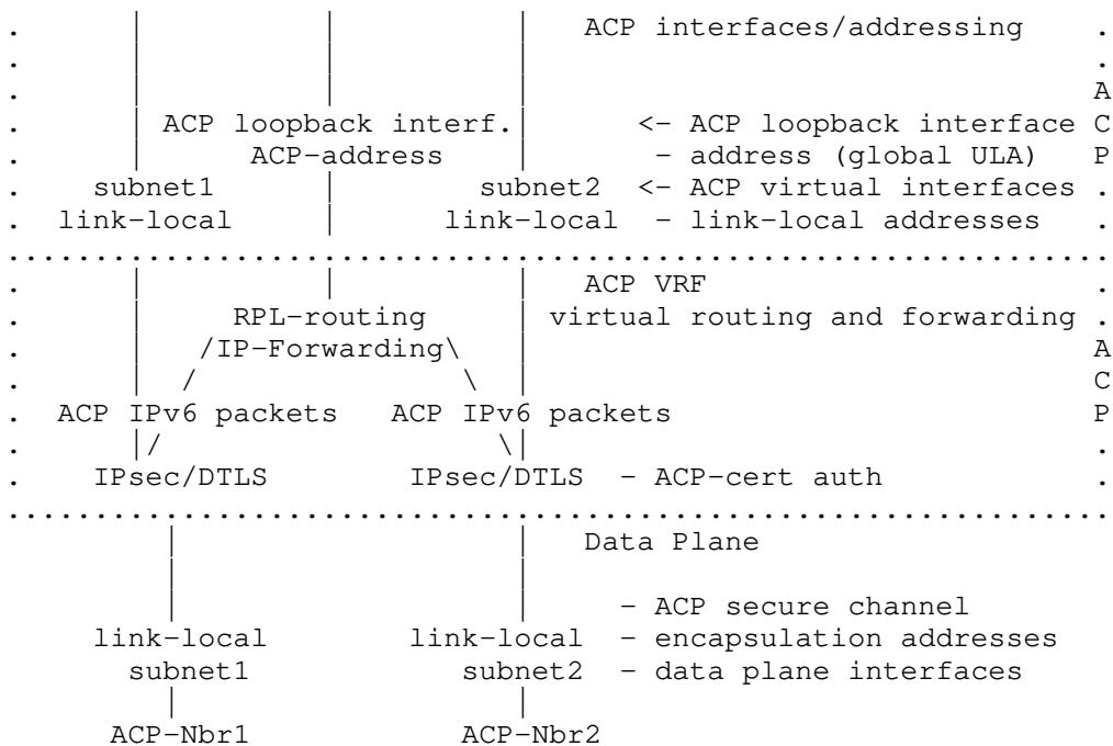
Figure 8: ACP as Security and Transport Substrate for GRASP
