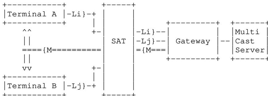
Figure 3: Network Architecture for a Reliable Multicast Using Network Coding
