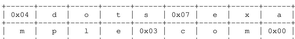
Figure 4: An Example of the dots-agent-name Encoding
