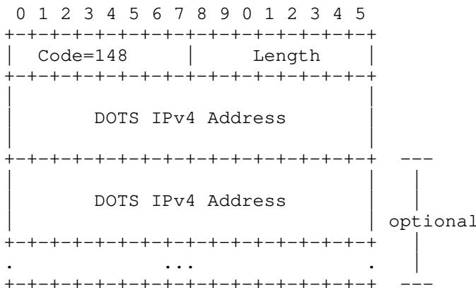
Figure 7: DHCPv4 DOTS Address Option
