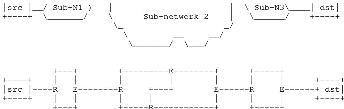
Figure 4: Replication and Elimination in Sub-networks for DetNet IP Networks
