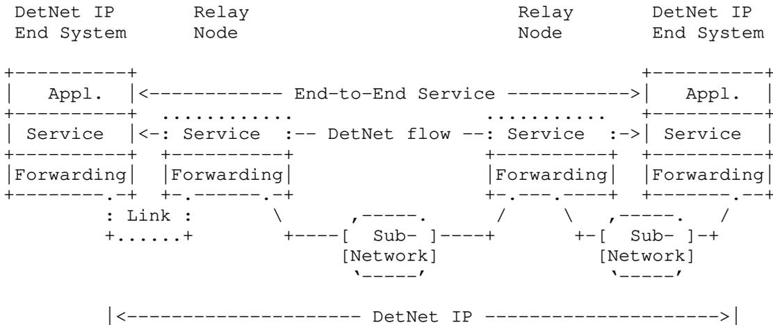
Figure 1: A Simple DetNet-Enabled IP Network
