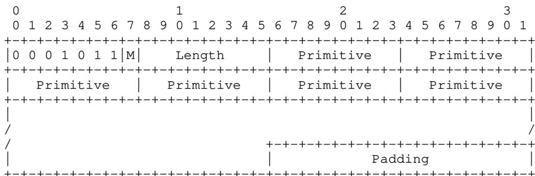
Figure 18: SUPPORTED-PRIMITIVES format
