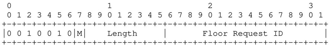
Figure 29: OVERALL-REQUEST-STATUS-HEADER format
