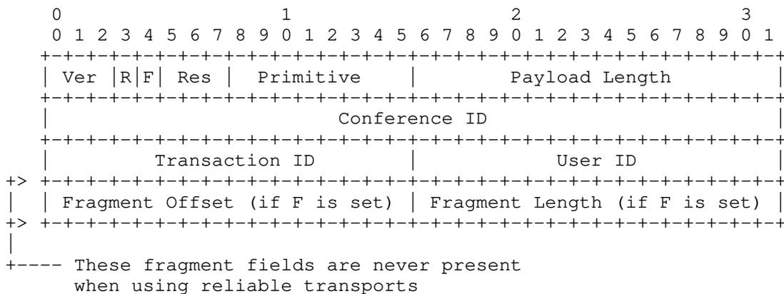
Figure 5: COMMON-HEADER format
