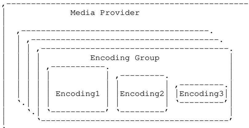
Figure 4: Encoding Group Structure
