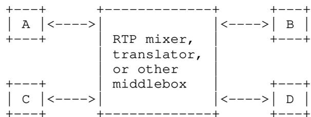
Figure 2: RTP Mixer with Only Unicast Paths
