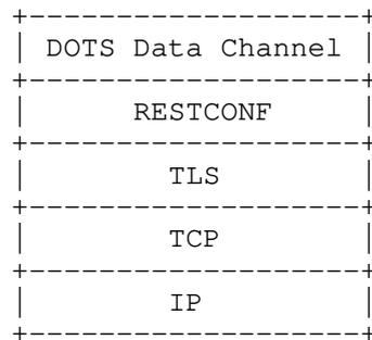
Figure 2: Abstract Layering of DOTS Data Channel
