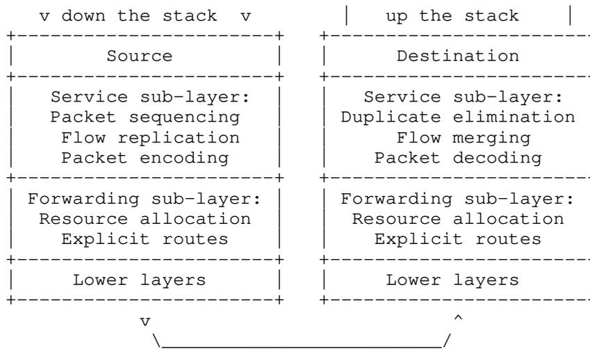
Figure 2: DetNet Data-Plane Protocol Stack
