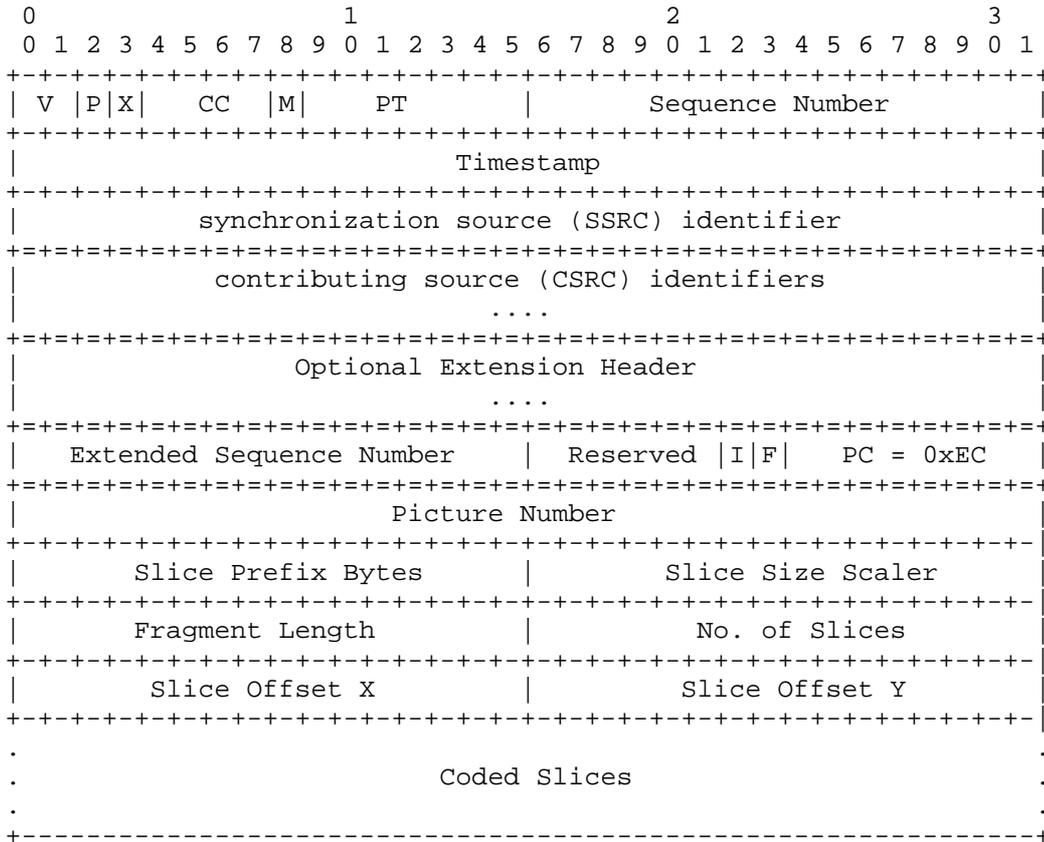
Figure 3: RTP Payload Format for Fragment Containing Slices
