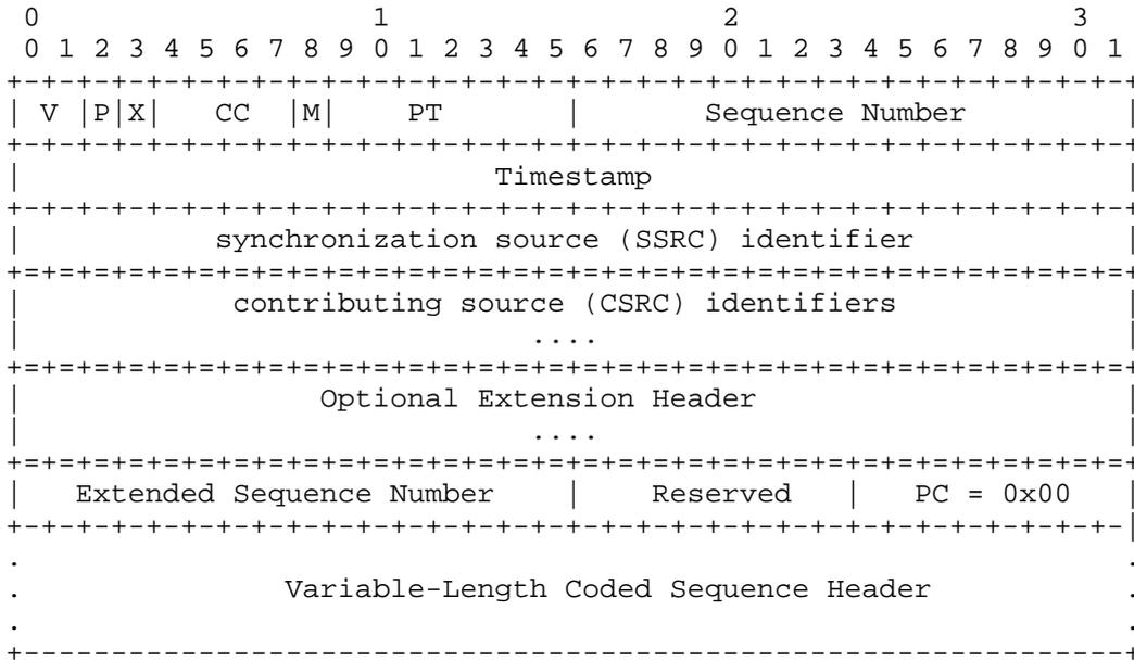
Figure 1: RTP Payload Format for Sequence Header
