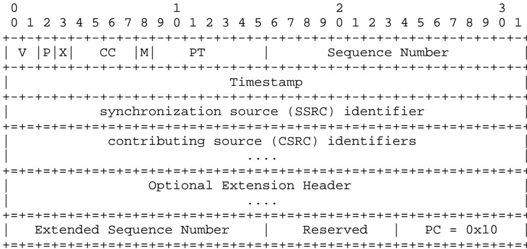
Figure 4: RTP Payload Format for End of Sequence
