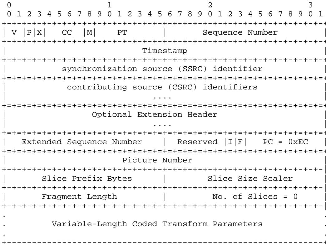
Figure 2: RTP Payload Format for Transform Parameters Fragment
