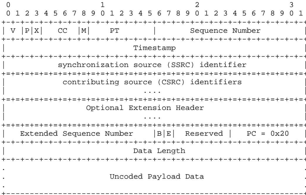
Figure 5: RTP Payload Format for Auxiliary Data
