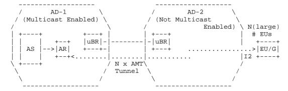
AS = multicast (e.g., content) Application Source uBR = unicast Border Router - not multicast enabled; otherwise, AR = uBR (in AD-1)
