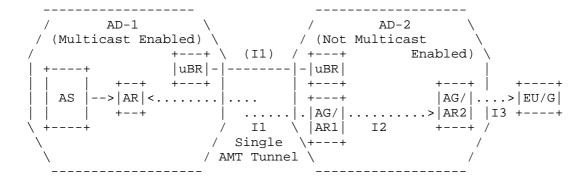
uBR = unicast Border Router - not multicast enabled; also, either AR = uBR (AD-1) or uBR = AGAR1 (AD-2)
