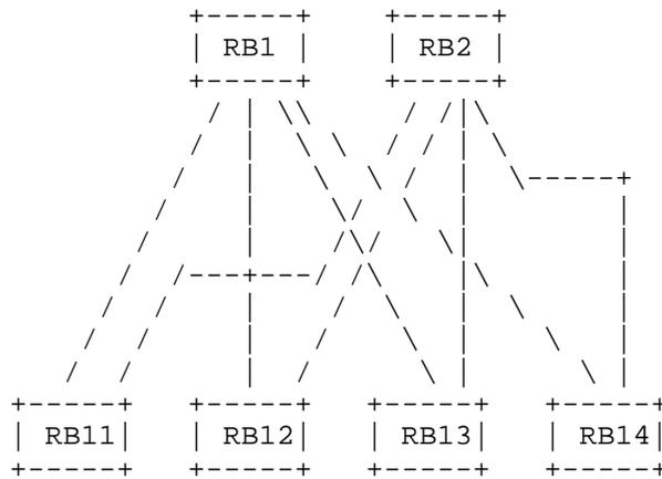
Figure 1: TRILL Network Based on Fat Tree Structure
