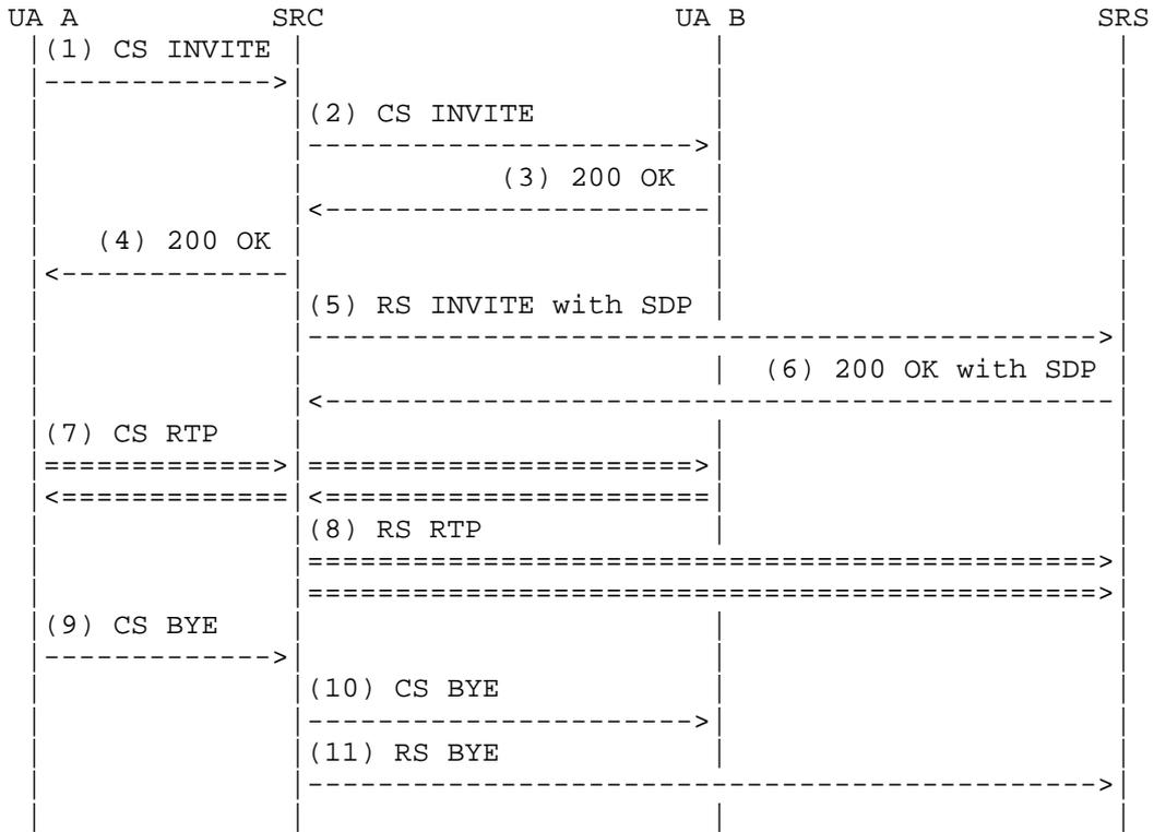
Figure 2: Basic Recording Call Flow with B2BUA as SRC
