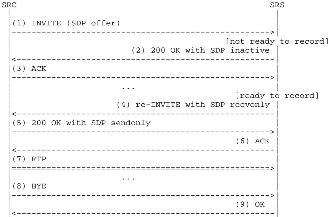
Figure 7: SRS Responding to Offer with a=inactive
