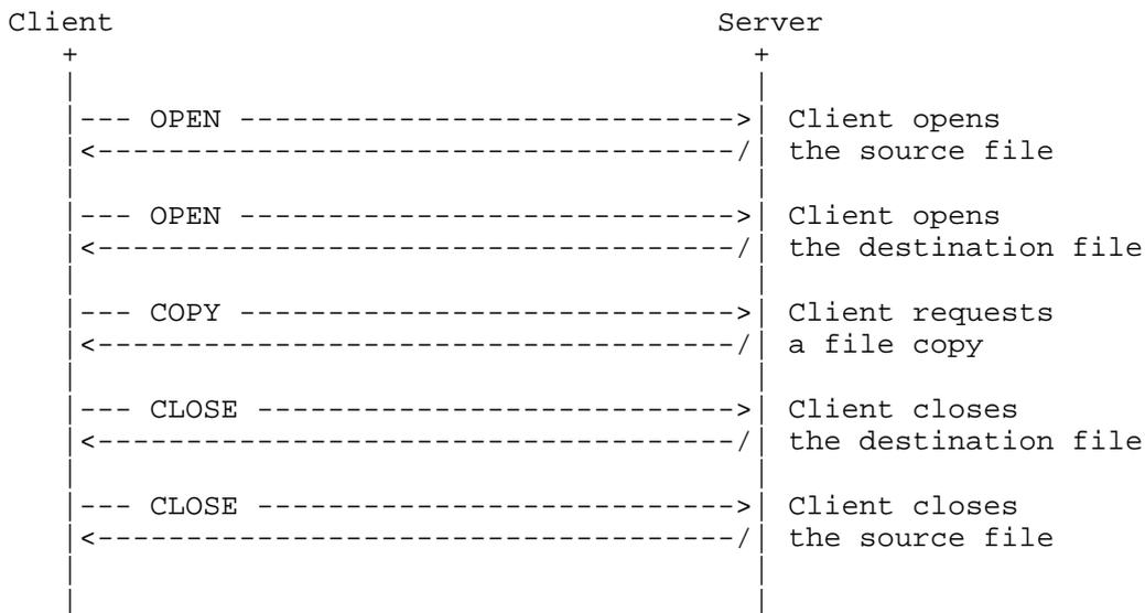
Figure 1: A Synchronous Intra-Server Copy
