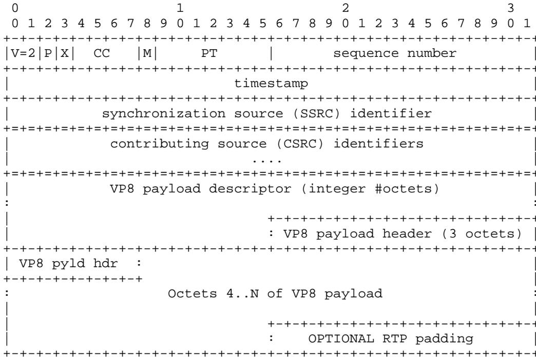
The VP8 payload descriptor and VP8 payload header will be described in Sections 4.2 and 4.3. OPTIONAL RTP padding MUST NOT be included unless the P bit is set. The figure specifically shows the format for the first packet in a frame. Subsequent packets will not contain the VP8 payload header and will have later octets in the frame payload.
