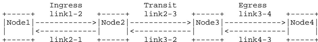
Figure 1: Path Computation in GMPLS Networks
