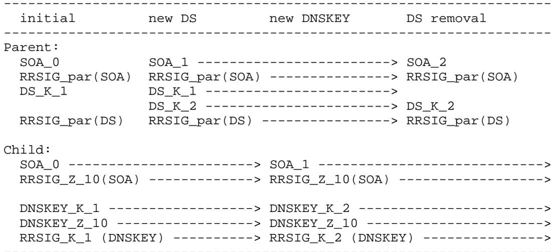
Figure 5: Stages of Deployment for a Double-DS Key Signing Key Rollover
