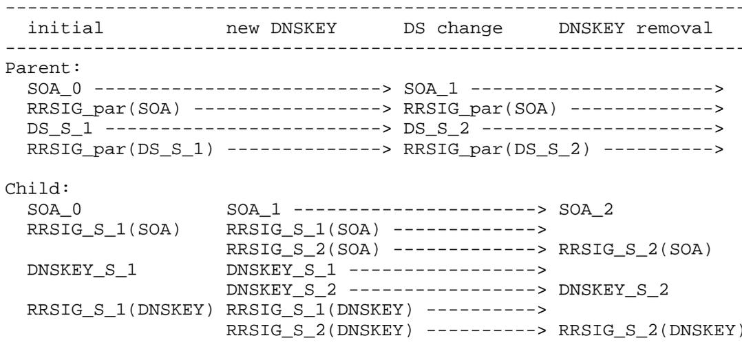
Figure 6: Stages of the Straightforward Rollover
