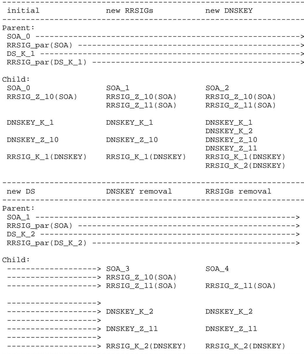
Figure 8: Stages of Deployment during an Algorithm Rollover
