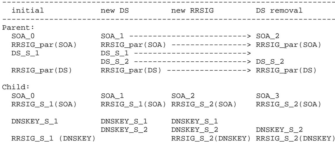
Figure 7: Stages of Deployment for a Double-DS Rollover in a Single-Type Signing Scheme
