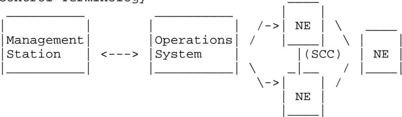
Network Elements use a Control/Signaling Communication Channel (SCC) for Transport of Signaling Information
