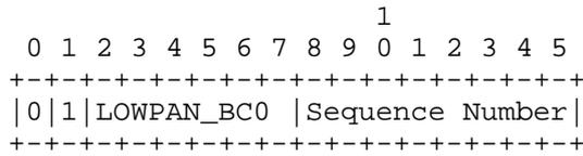
Figure 11: Broadcast Header
