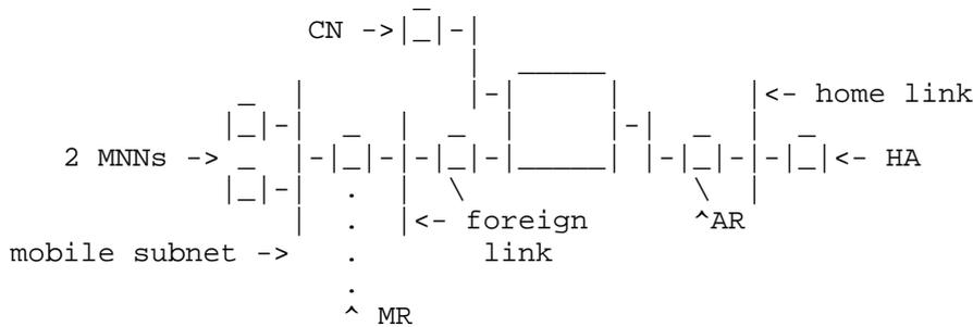
Figure 2: Single Mobile Subnet on a Foreign Link
