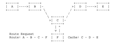
The concatenation of the accumulated route record from the Route Request and the cached route from F's Route Cache would include a duplicate node in passing from C to F and back to C.
