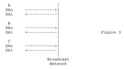
The problem can be solved by using the same SA parameters (SPI, keys, etc.) for both inbound (SAi) and outbound (SAo) SAs as shown in Figure 3.
