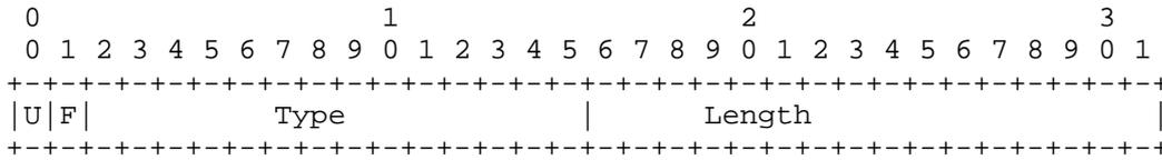
The type field for the SONET/SDH Traffic Parameters TLV is: 0x0838.
