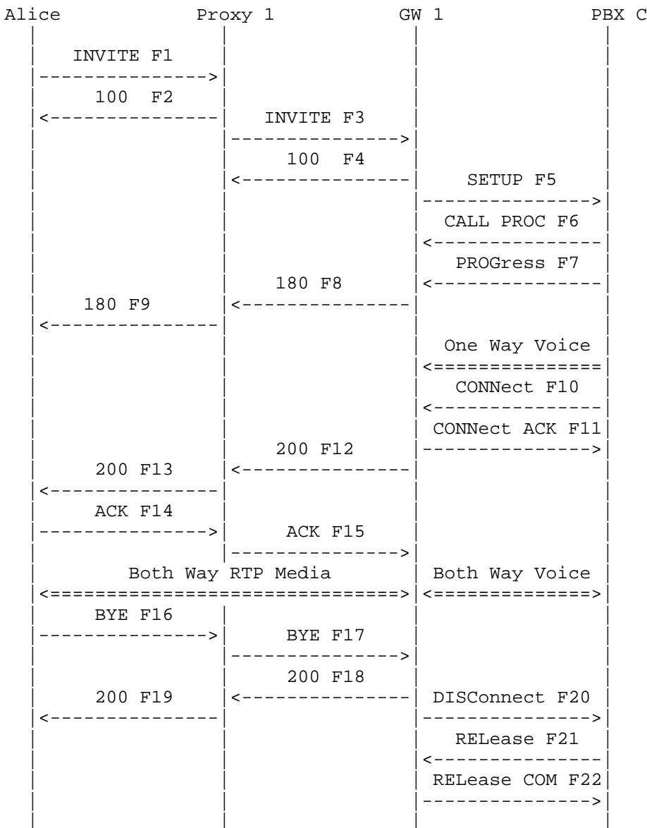
Alice is a SIP device while Carol is connected via a Gateway (GW 1) to a PBX. The PBX connection is via a ISDN trunk group. Alice dials Carol's telephone number (918-555-3333) which is globalized and put into a SIP URI.
