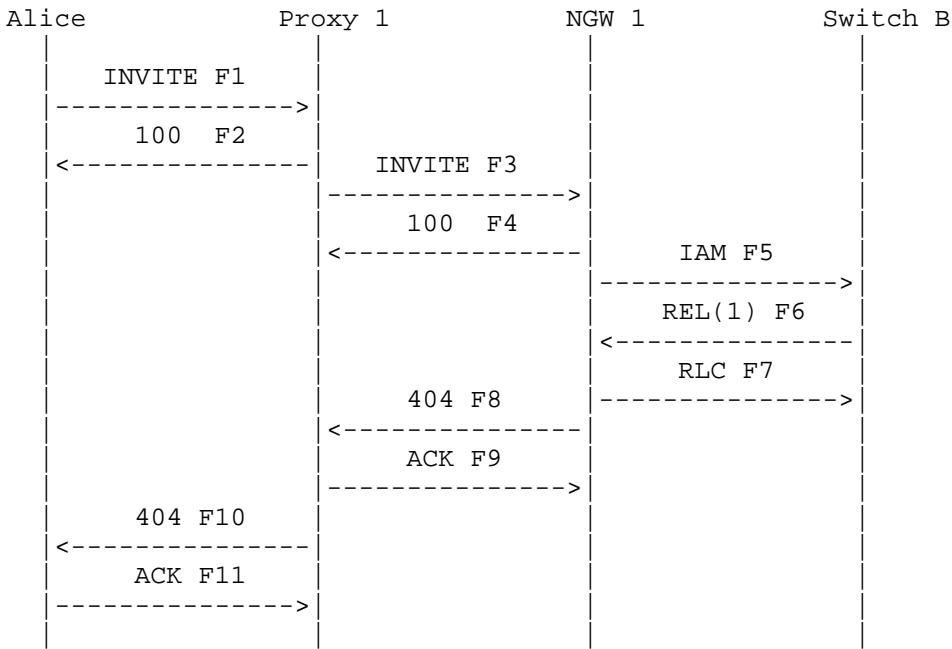
Alice calls PSTN Bob through a Proxy Server Proxy 1 and a Network Gateway NGW 1. The call is rejected by the PSTN with a ANSI ISUP Release message REL containing a specific Cause code. This cause value (1) is mapped by the Gateway to a SIP 404 Address Incomplete response which is proxied back to Alice. For more details of ISUP cause value to SIP response mapping, refer to [4].
