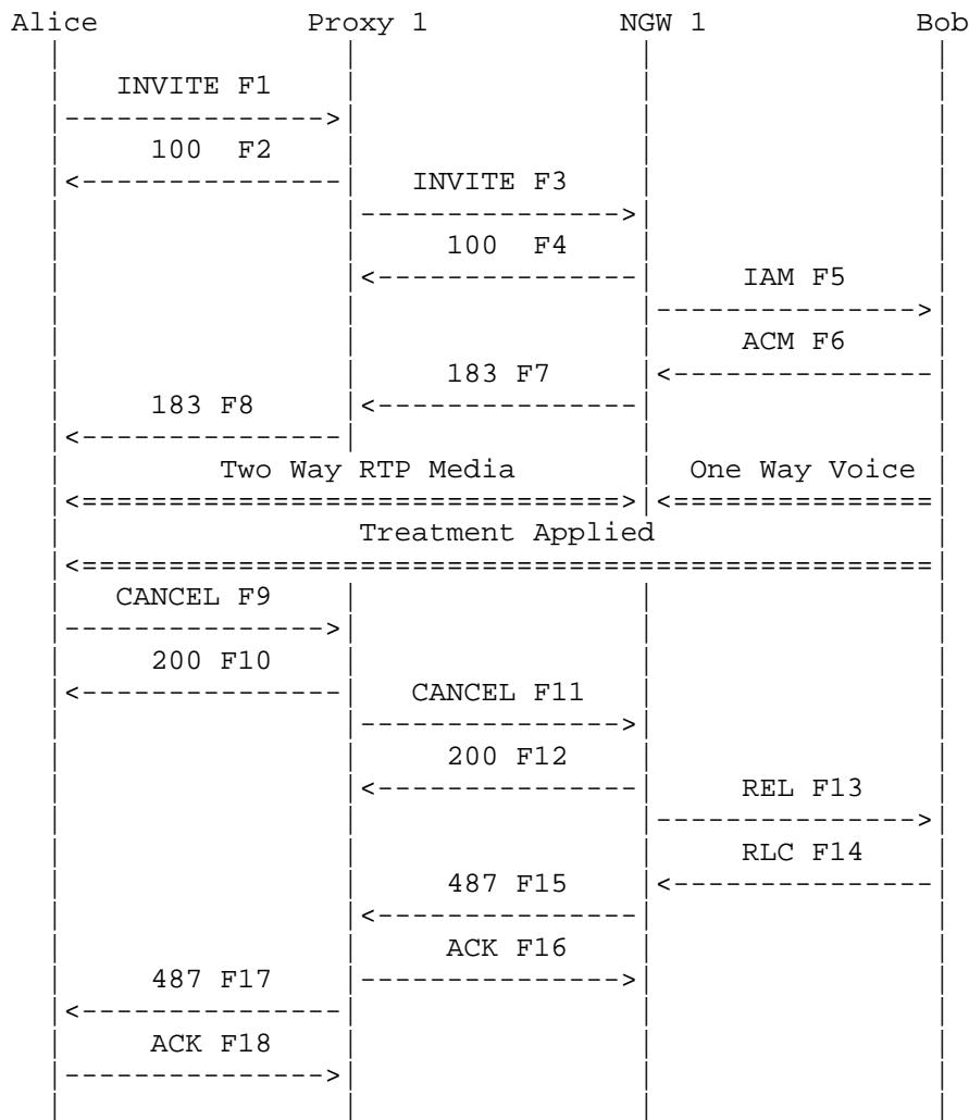
Alice calls Bob in the PSTN through a proxy server Proxy 1 and a Network Gateway NGW 1. The call is rejected by the PSTN with an in-band treatment (tone or recording) played. Alice hears the treatment and then hangs up, which results in a CANCEL (F9) being sent to terminate the call. (A BYE is not sent since no final response was ever received by Alice.)
