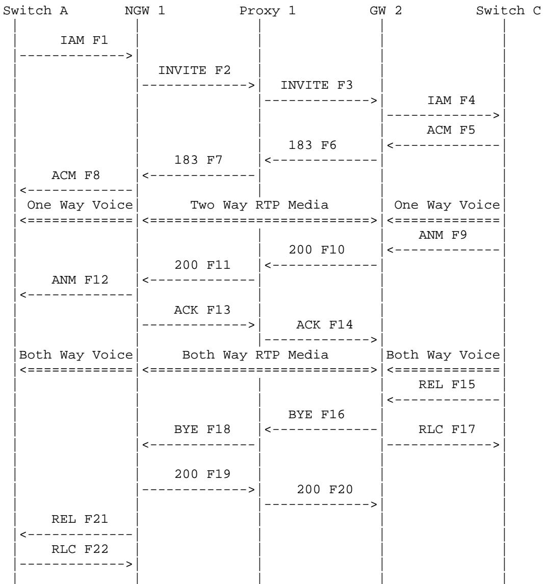
In this scenario, Alice in the PSTN calls Carol who is an extension on a PBX. Alice's telephone switch signals via SS7 to the Network Gateway NGW 1, while Carol's PBX signals via SS7 with the Gateway GW 2. The CdPN and CgPN are mapped by GW 1 into SIP URIs and placed in the To and From headers. Proxy 1 looks up the dialed digits in the Request-URI and maps the digits to the PBX extension of Carol, which
