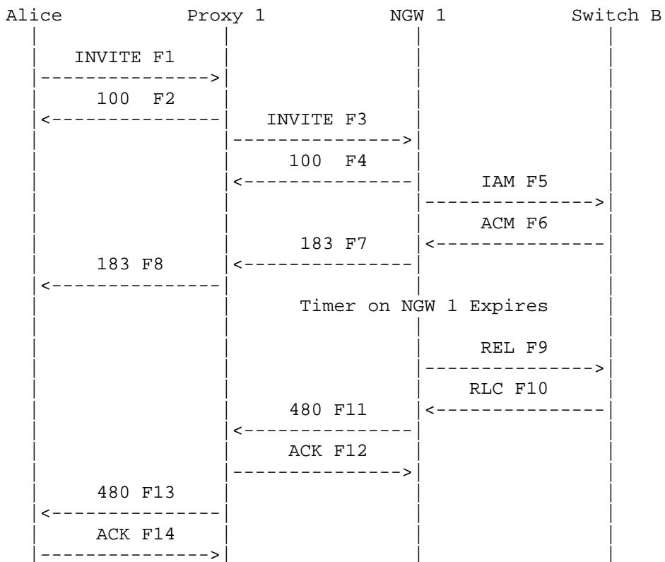
Alice calls Bob in the PSTN through a proxy server Proxy 1 and Network Gateway NGW 1. The call is released by the Gateway after a timer expires due to no ANswer Message (ANM) being received. The Gateway sends an ISUP Release REL message to the PSTN and a 480 Temporarily Unavailable response to Alice in the SIP network.
