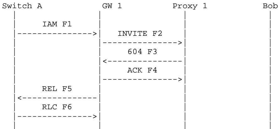
Alice attempts to place a call through Gateway GW 1 and Proxy 1, which is unable to find any routing for the number. The call is rejected by Proxy 1 with a REL message containing a specific Cause value mapped by the gateway based on the SIP error.
