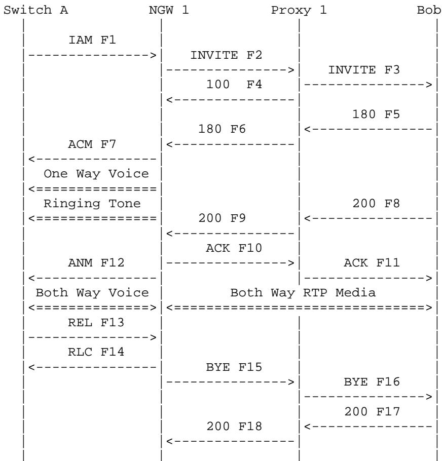
In this scenario, Alice from the PSTN calls Bob through a Network Gateway NGW1 and Proxy Server Proxy 1. When Bob answers the call, the media path is setup end-to-end. The call terminates when Alice hangs up the call, with Alice's telephone switch sending an ISUP RERelease message that is mapped to a BYE by NGW 1.
