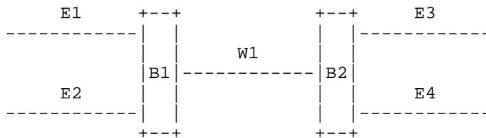
E1, E2, E3, and E4 are Ethernet LANs (or Token Ring, FDDI, etc.). W1 is a WAN (PPP over T1). B1 and B2 are MAC level bridges.
