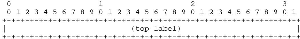
The contents of a LABEL is a single label, encoded in 4 octets. Each generic MPLS label is an unsigned integer in the range 0 through 1048575. Generic MPLS labels and FR labels are encoded right aligned in 4 octets. ATM labels are encoded with the VPI right justified in bits 0-15 and the VCI right justified in bits 16-31.
