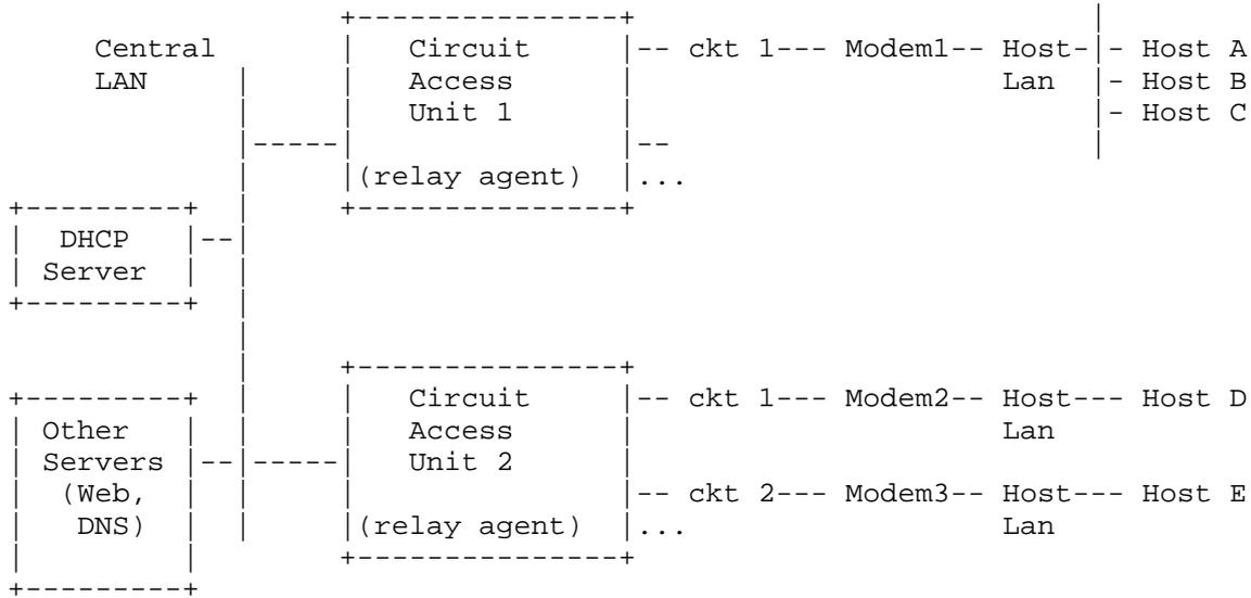
Figure 1: DHCP High Speed Circuit Access Model
