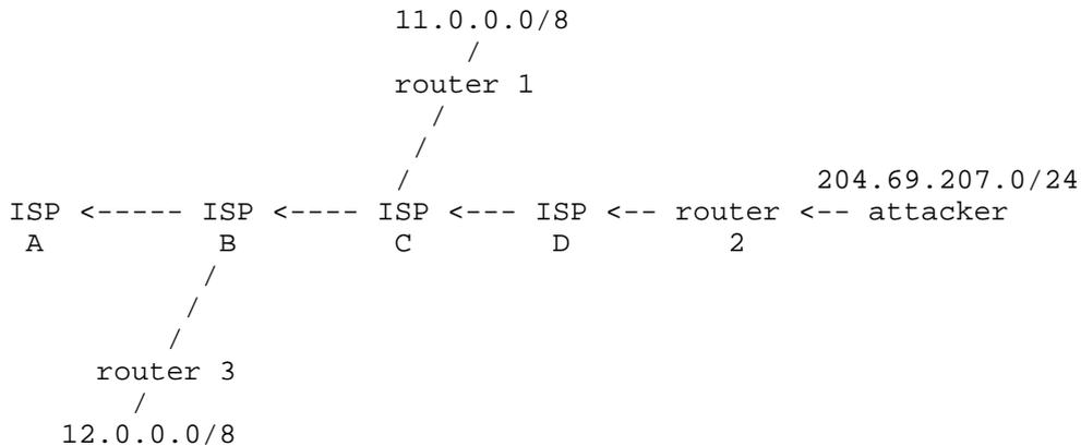
In the example above, the attacker resides within 204.69.207.0/24, which is provided Internet connectivity by ISP D. An input traffic filter on the ingress (input) link of "router 2", which provides connectivity to the attacker's network, restricts traffic to allow only traffic originating from source addresses within the 204.69.207.0/24 prefix, and prohibits an attacker from using "invalid" source addresses which reside outside of this prefix range.
