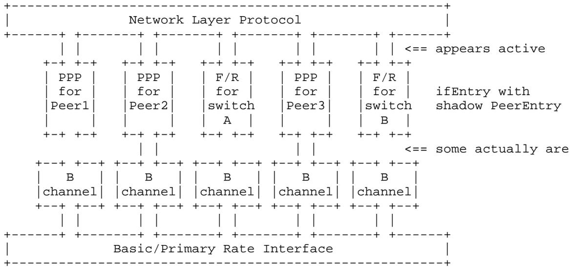
Mapping of IP interfaces to Called Peers to B Channels
