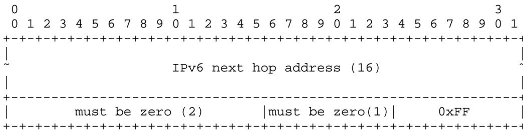
Specifying a value of 0:0:0:0:0:0:0:0 in the prefix field of a next hop RTE indicates that the next hop address should be the originator of the RIPng advertisement. An address specified as a next hop must be a link-local address.
