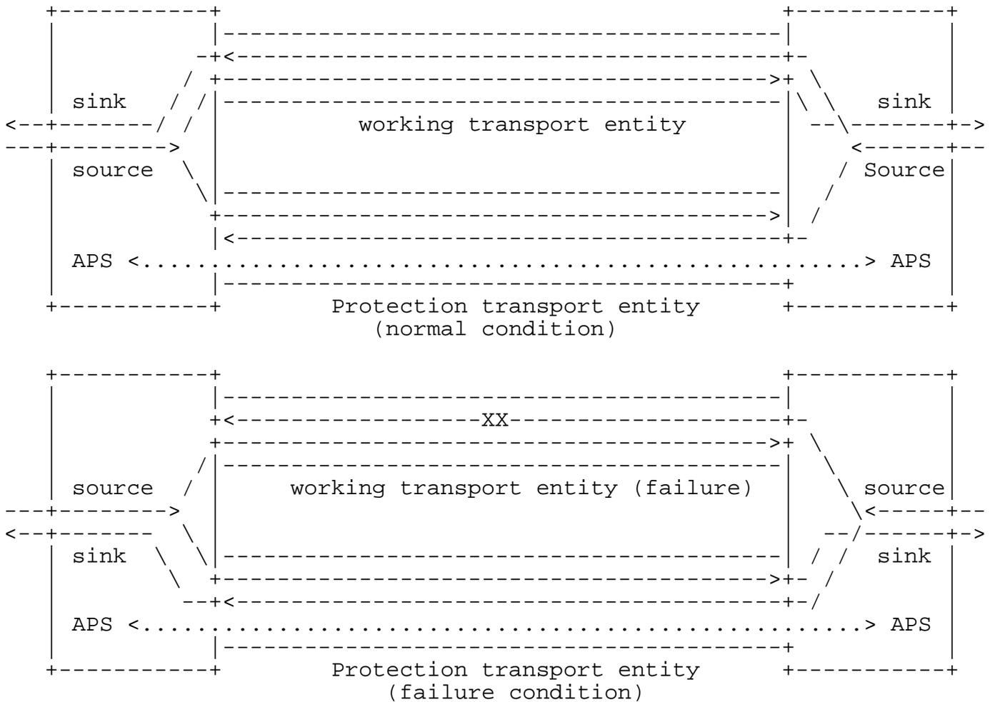
Figure 2 1+1 Bidirectional Linear Protection Switching
