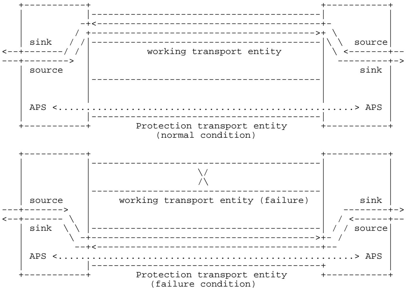
Figure 3 1:1 Bidirectional Linear Protection Switching
