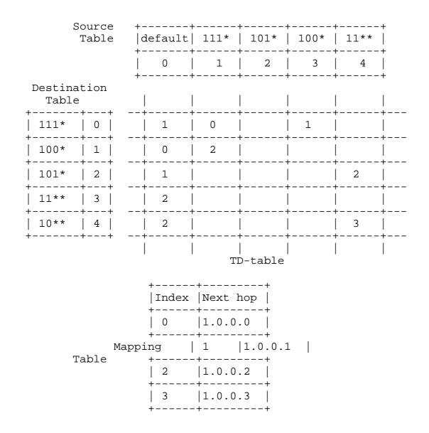
Figure 4: Forwarding Table for TwoD-IP
