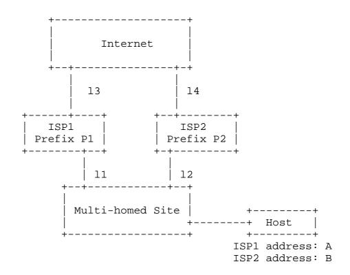
Figure 1: TwoD-IP routing for multi-homing
