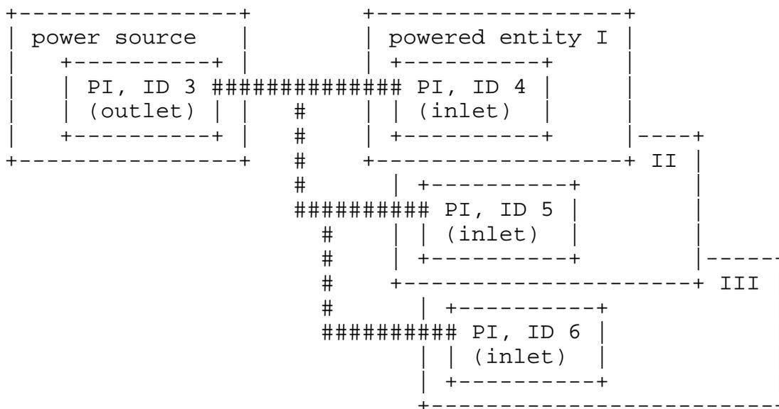
Figure 9: PSU Layer for a Single PS Supplying Multiple PEs.
