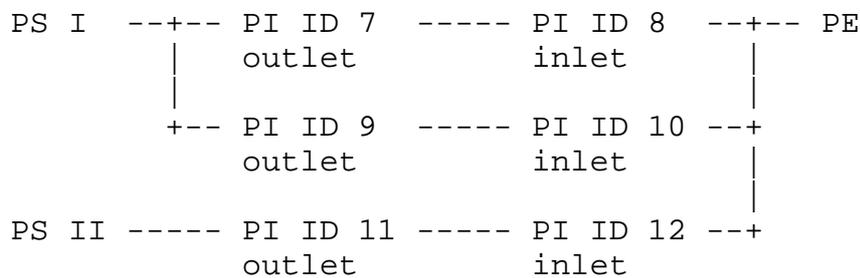
Figure 11: Multiple Power Supply for Single Powered Device
