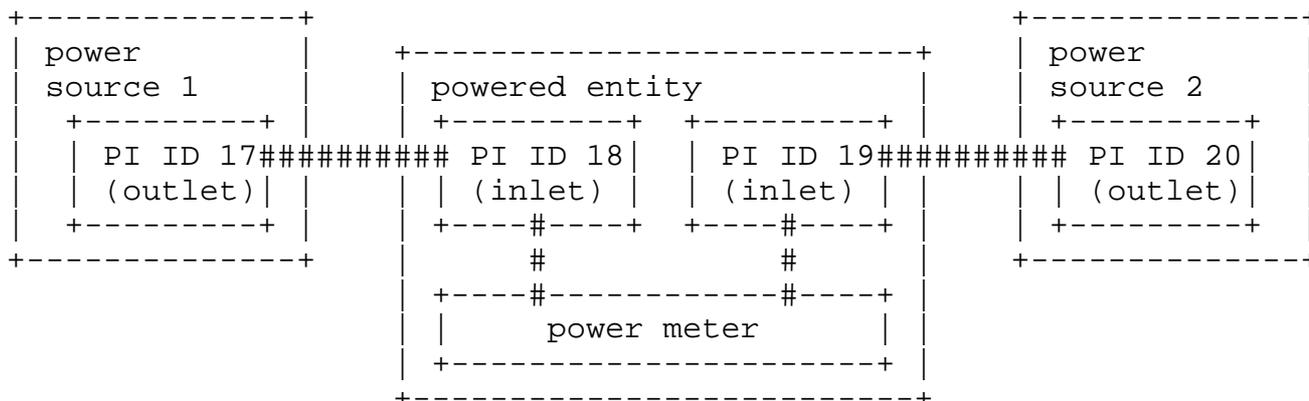
Figure 14: Dual power supply topology
