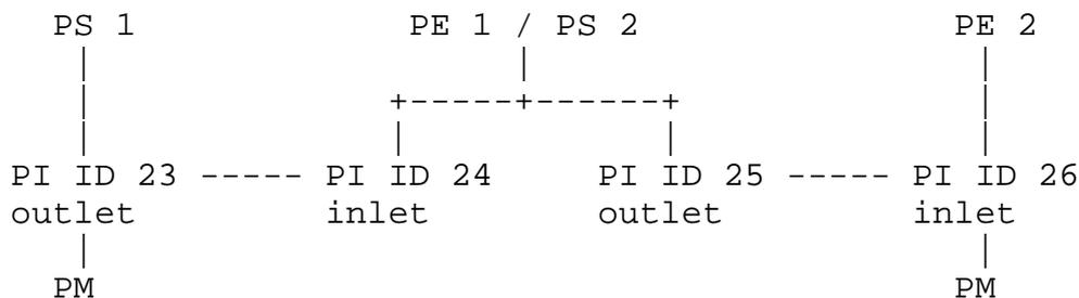
Figure 18: Relationships between Cascaded Power Sources
