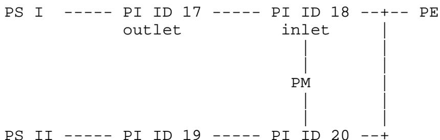
Figure 15: PSU Layer Model of a Dual Role Power Source
