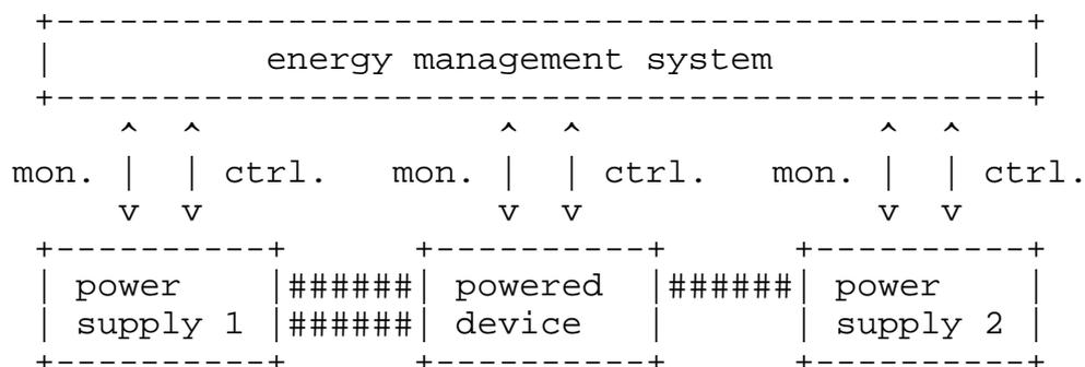
Figure 5: Multiple Power Supply for Single Powered Device
