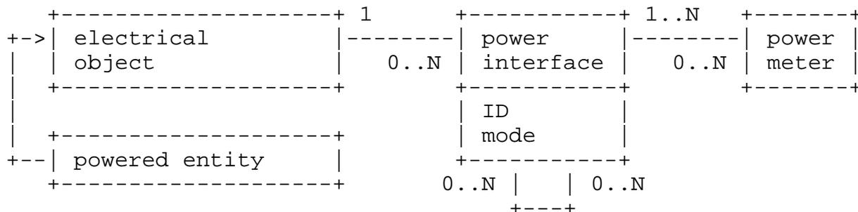
Figure 19: Basic Information Model of the PSU Layer
