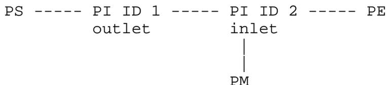
Figure 8: PSU layer model for one-to-one supply topology
