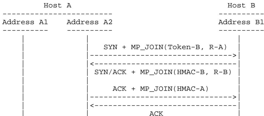
HMAC-A = HMAC(Key=(Key-A+Key-B), Msg=(R-A+R-B))
