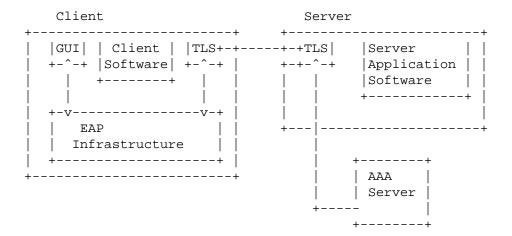
The above diagram shows the typical deployment. The client has software that either includes a UI for some EAP methods, or else is able to invoke some operating system EAP infrastructure that takes care of the user interaction. The server is configured with the address and protocol of the AAA server. Typically the AAA server communicates using the RADIUS protocol with EAP ([RADIUS] and [RAD-EAP]), or the Diameter protocol ([Diameter] and [Dia-EAP]).
