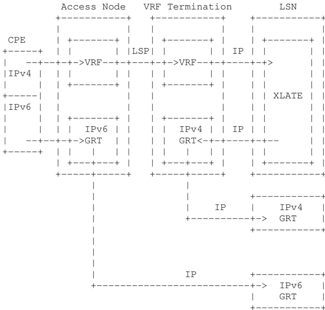
Figure 3 NAT44/LSN with IPv6 Dual Stack Operation
