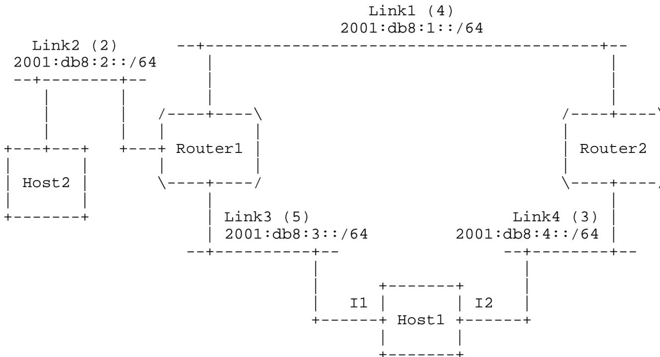
The figure shows two routers (Router1, Router2) and two hosts (Host1, Host2). These nodes are connected to each other through 4 links (Link1, Link2, Link3, Link4). The values in brackets represent the corresponding link costs. Also, Host1 is a multiple interfaces device: it is connected to Link3 via its network interface I1 and to link4 via its network interface I2.
