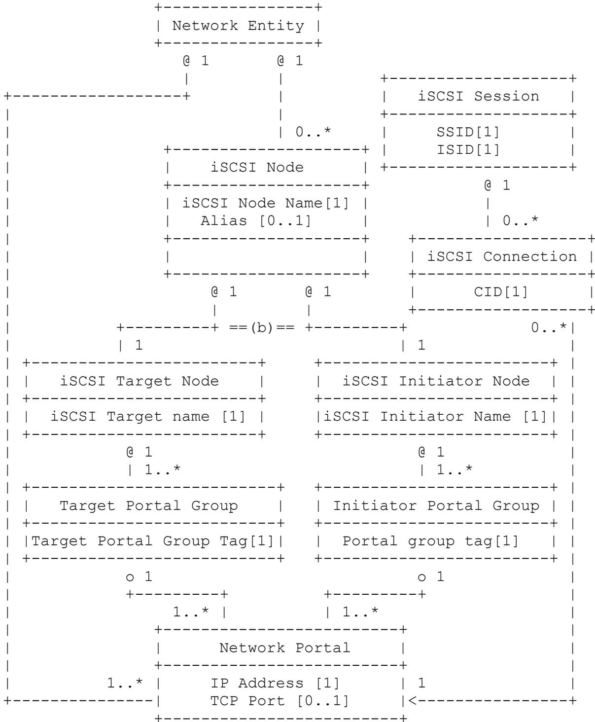
(b) Each instance of an iSCSI Node class MUST contain one iSCSI Target Node instance or one iSCSI Initiator Node instance, or both. However, in all scenarios, note that an iSCSI Node MUST only have a single iSCSI Name. Note the related requirement in Section 4.2.7.1.
