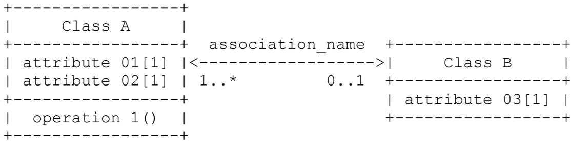
The preceding diagram is an example where Class A knows about Class B (i.e., read as "Class A association\_name ClassB") and Class B knows about Class A (i.e., read as "Class B association\_name Class A"). The use of association\_name is optional. The multiplicity notation (1..\* and 0..1) indicates the number of instances of the object.
