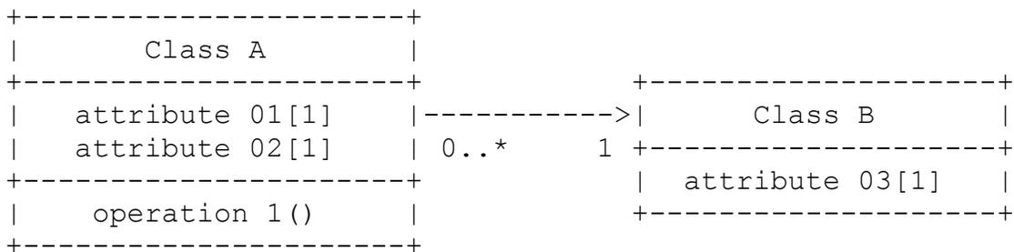
The preceding diagram is an example where Class A knows about Class B (i.e., read as "Class A knows about Class B") but Class B does not know about Class A.
