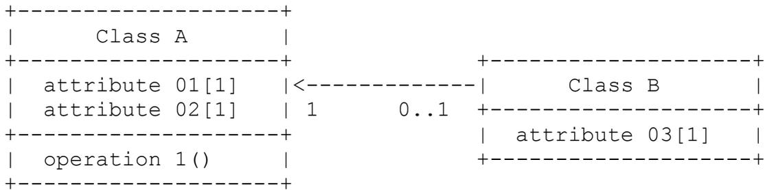
The preceding diagram is an example where Class B knows about Class A (i.e., read as "Class B knows about Class A") but Class A does not know about Class B.
