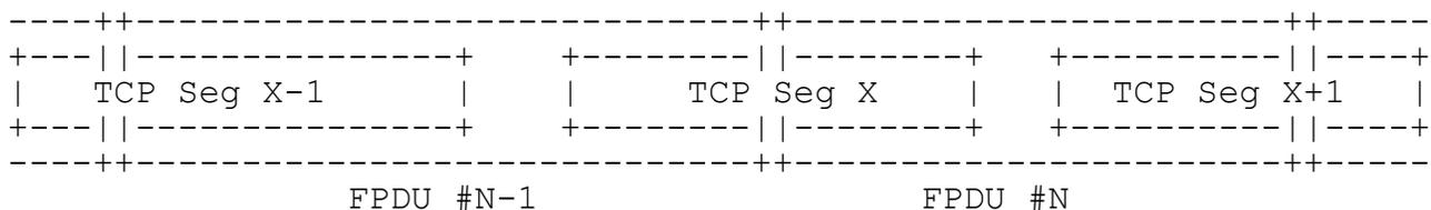
Figure 10: Non-aligned FPDU freely placed in TCP octet stream
