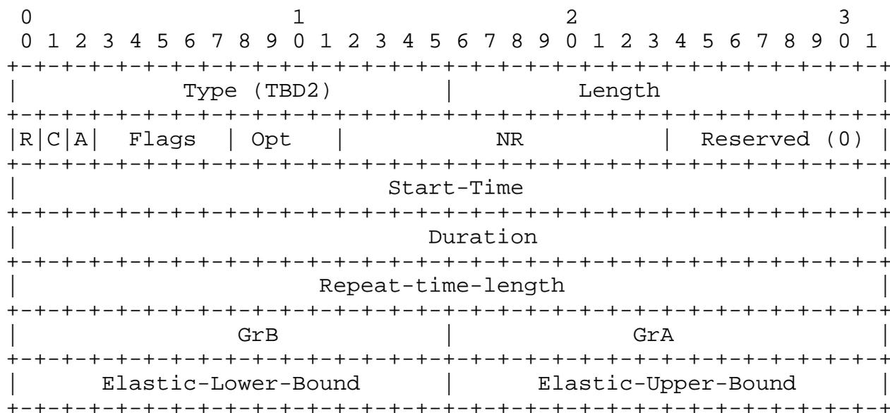
The type of the TLV is [TBD2] and the TLV has a fixed length of 24 octets. The description, format and meaning of the Flags (R, C and A bit), Start-Time, Duration, GrB, GrA, Elastic-Lower-Bound and Elastic-Upper-Bound fields remains same as SCHED-LSP-ATTRIBUTE TLV.
