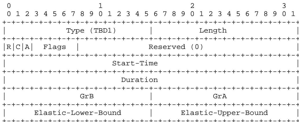
The type of the TLV is [TBD1] and the TLV has a fixed length of 20 octets.
