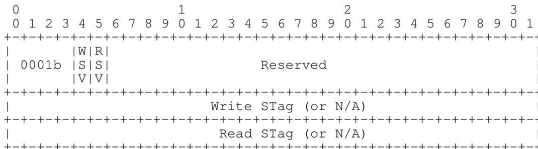
Figure 3 iSER Header Format for iSCSI Control-Type PDU
