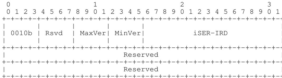
Figure 4 iSER Header Format for iSER Hello Message
