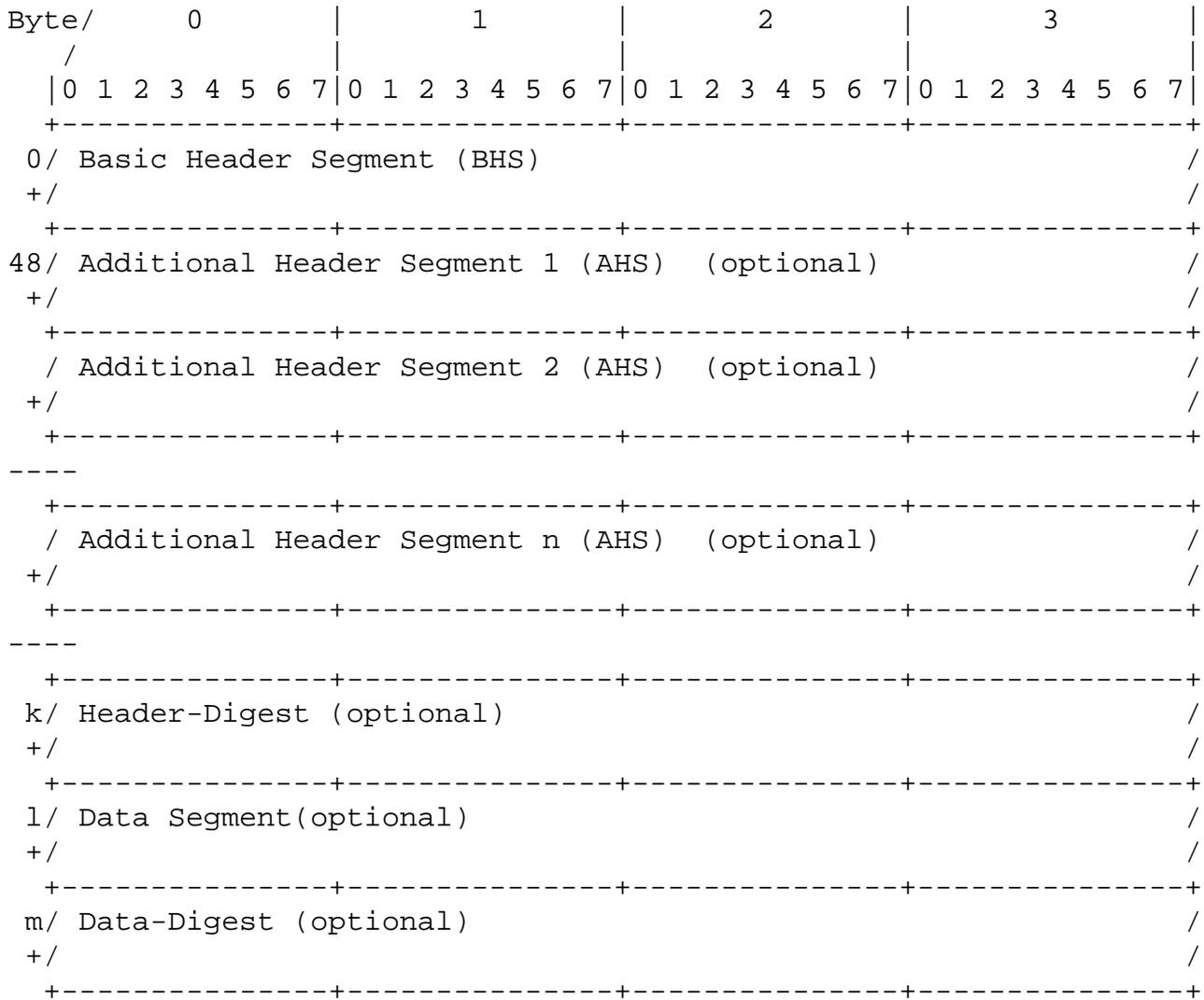
All PDU segments and digests are padded to the closest integer number of four byte words. For example, all PDU segments and digests start at a four byte word boundary and the padding ranges from 0 to 3 bytes. The padding bytes SHOULD be sent as 0.
