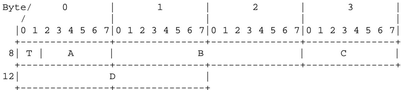
The T field identifies the format and usage of A, B, C, and D as indicated below:
