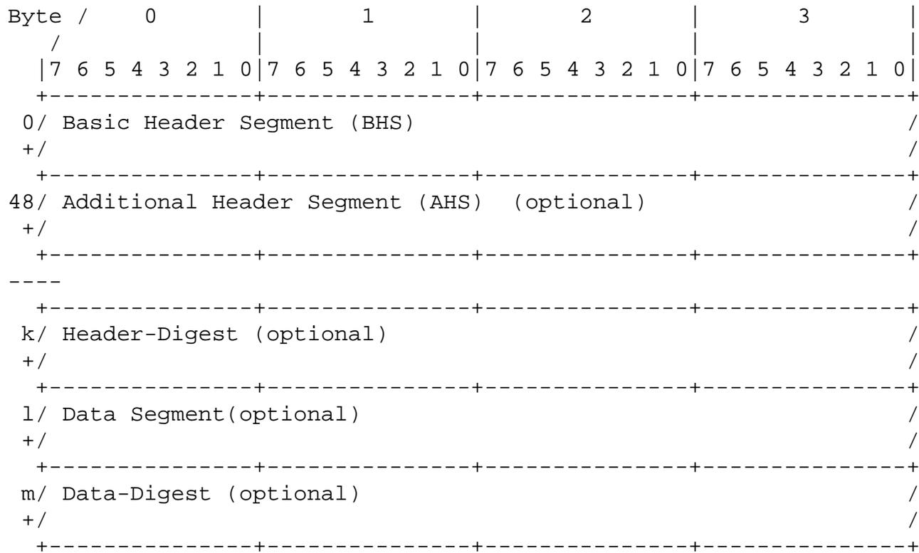
All PDU segments and digests are padded to an integer number of four byte words. The padding bytes SHOULD be sent as 0.
