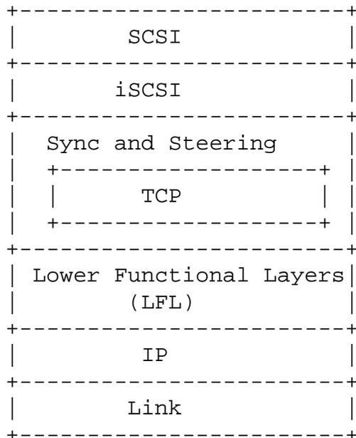
In this model, LFL can be IPsec (a mechanism changing the IP stream and invisible to TCP). We assume that Sync and Steering operates just underneath iSCSI. An implementation may choose to place Sync and Steering somewhere else in the stack if it can translate the information kept by iSCSI in terms valid for the chosen layer.
