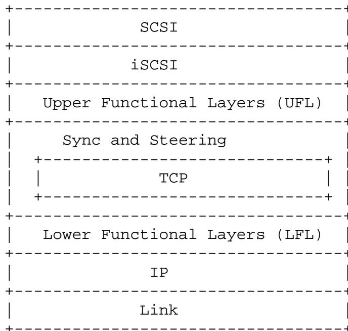
In this model, UFL can be TLS (see[RFC2246]) or some other transport conversion mechanism (a mechanism that changes the TCP stream, but that is transparent to iSCSI).
