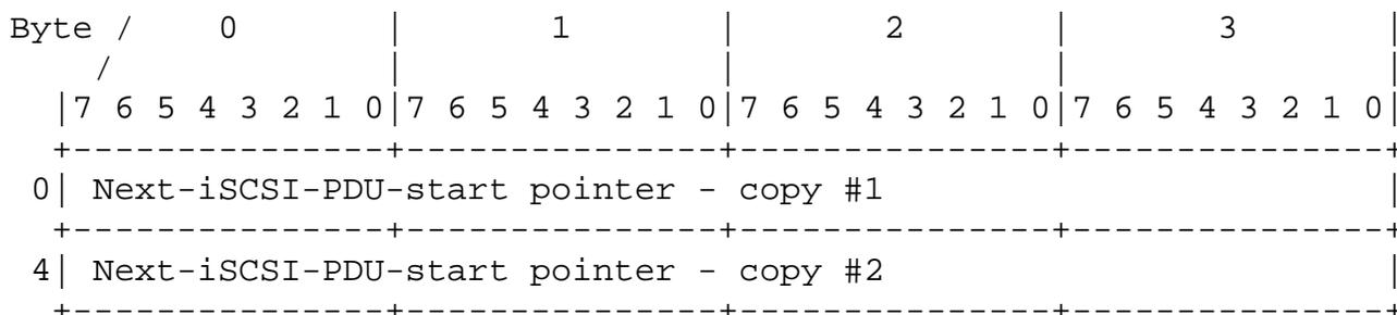
The Marker schemes uses payload byte stream counting that includes every byte placed by iSCSI in the TCP stream except for the markers themselves. It also excludes any bytes that TCP counts but are not originated by iSCSI.
