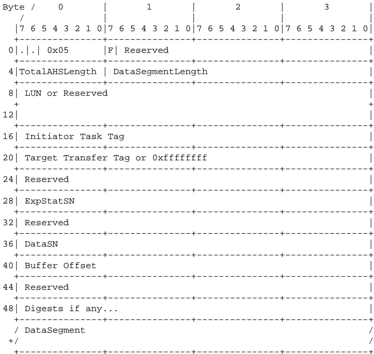
The SCSI Data-in PDU for READ operations has the following format:
