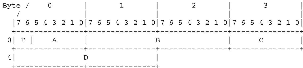
The T field identifies the format and usage of A, B, C & D as indicated below:
