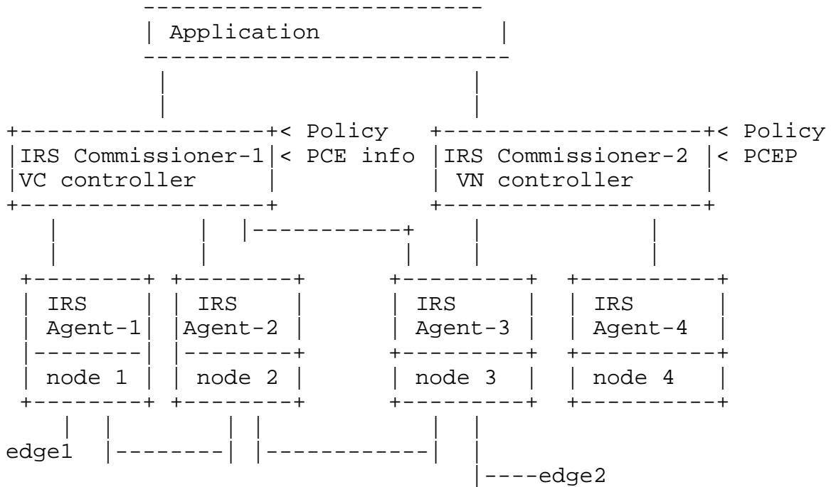
While the set-up of these virtual circuits is possible with current technology, the lack of the IRS-like framework makes VCoD network complex. With this support, VCoD may be able to reduce complexity on the individual nodes.
