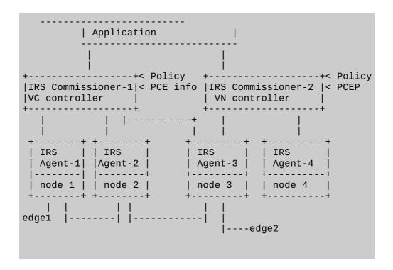
While the set-up of these virtual circuits is possible with current technology, the lack of the IRS-like framework makes VCoD network complex. With this support, VCoD may be able to reduce complexity on the individual nodes.
