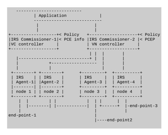
This topology shares some configuration needs with the central membership computation for MPLS VPNs from (draft-white-irs-use-cases) but the mechanisms are not specific to MPIS VPNS.
