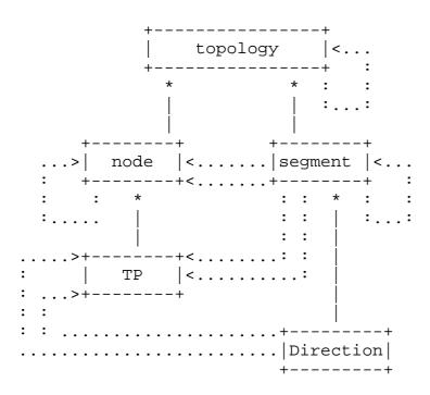
The basic information model works as follows: A service topology contains service nodes and segments. A segment connects two nodes (a source and a destination) and have direction, may be unidirectional or bidirectional. unidirectional is one where traffic is passed through a set of SF nodes in one forwarding direction only. Bidirectional is one where traffic is passed through a set of SF nodes in both
