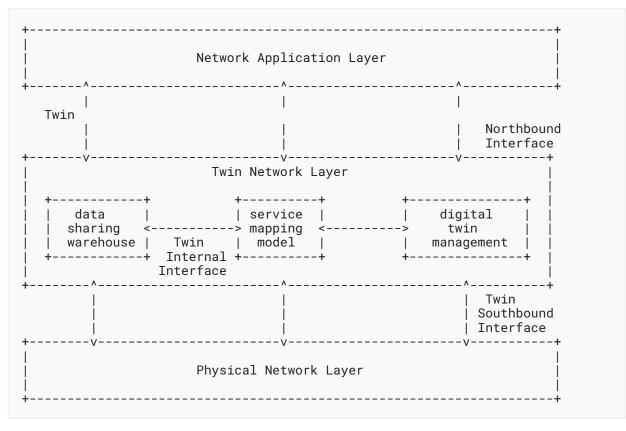
Figure 1: Schematic Representation of DTN Interface
