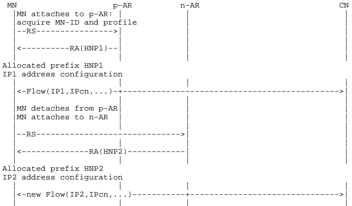
Figure 4. A flow uses the IP allocated from the network at which the MN is attached when the flow is initiated.
