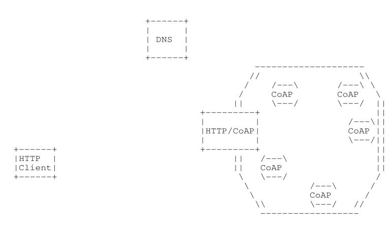
Figure 1: Server-side HC proxy deployment scenario
