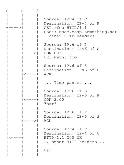
Figure 2: HTTP/IPv4 to CoAP/IPv6 mapping
